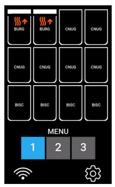
Each recipe is programmed with a "hold time". The hold time can be configured for any time between 1 minute to 540 minutes. Pressing on any well will start the timer.
