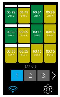
When a well is started the color of the well will change to green, use this product first. When the second well of the same recipe is started the started well change to amber, use this next. When subsequent wells of the same recipe are started, they will also be amber. If a different well is started with a different recipe and there is no other well running with the recipe - then it will also have green background.
