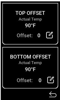
When this screen appears the TOP and BOTTOM current temperature offset value will appear. The actual temperature read from the RFHU for both the top and bottom heaters will also appear.
